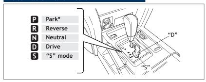
\* The "ENGINE START STOP" switch must be in IGNITION ON mode and the brake pedal depressed to shift from Park.
